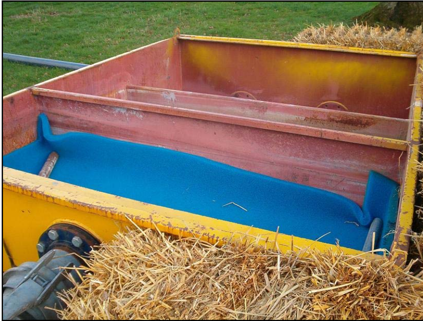
Figure A7 - Photograph of a typical settlement tank showing the hose at the entry point to the tank and the baffle plates. The blue foam shown can be added to the tank to capture solids at the entry point for flows. This size tank is supplied by 75mm and 100mm pumpsets only.
